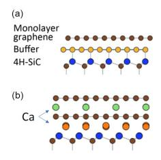
Figure 1. Schematic structure of (a) as-grown and (b) Ca-intercalated epitaxial graphene on SiC.
