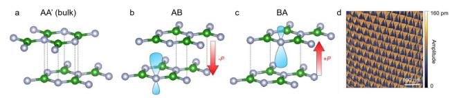
Figure 1. (a) Crystal structure of bulk hexagonal boron nitride and (b, c) parallel-stacked boron nitride.(d) Ferroelectric moiré lattice observed with piezoresponse force microscopy. Adapted from [2].
