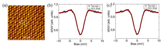
**Figure 1. (a)** Atomic-scale STM image of the C<sub>6</sub>CaC<sub>6</sub> taken at 4.2 K with  $V_s = -110$  mV, I = -80 pA. **(b)** Averaged tunneling spectrum taken at 4.2 K with  $V_s = 10$  mV, I = 100 pA,  $\Delta = 1.92$  meV. The red line is the fitting result to the Dynes function. **(c)** Temperature dependence of real part mutual inductance  $V_P^{\text{Re}}$  collected at various magnetic fields.
